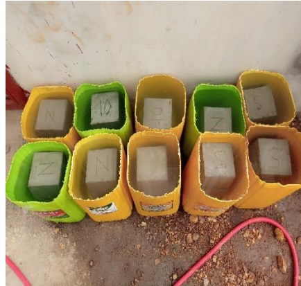
(b)Curing of specimens
