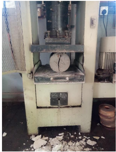
(c) Load applied to cylinder until failure
