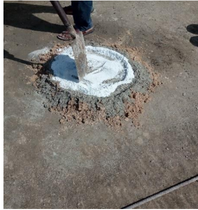
(b) Cement and recycled glass powder added to fine aggregates
