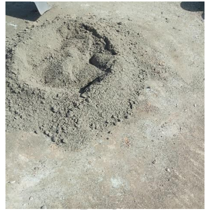
(c) Mixture of cement, recycled glass powder and fine aggregates
