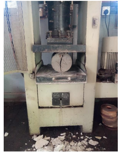
(c) Load applied to cylinder until failure
