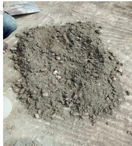
(e) Mixture of fine aggregate, cement, recycled glass powder, coarse aggregate and palm kernel shells
