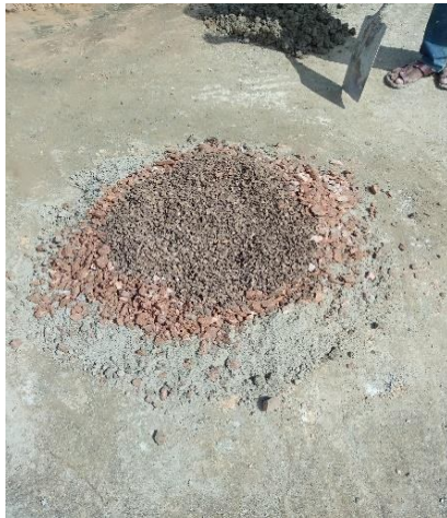
(d) Coarse aggregate and Palm kernel shells added to the mixture of cement, recycled glass powder and fine aggregate
