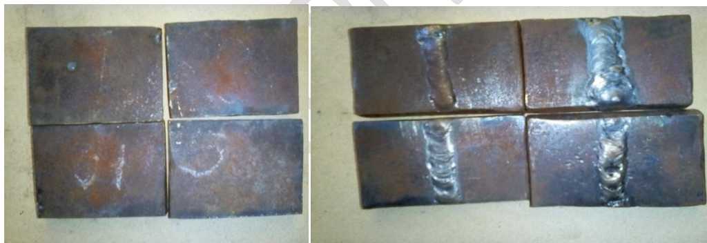
Figure 1a: Sample of Mild Steel Plate of IS2062 E-250 and its Welding Samples
