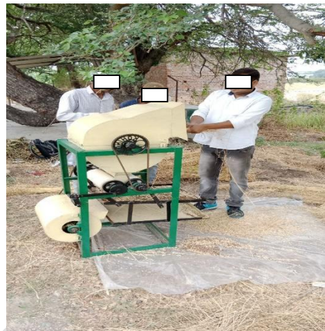
Fig.2. Threshing of linseed crop by thresher
