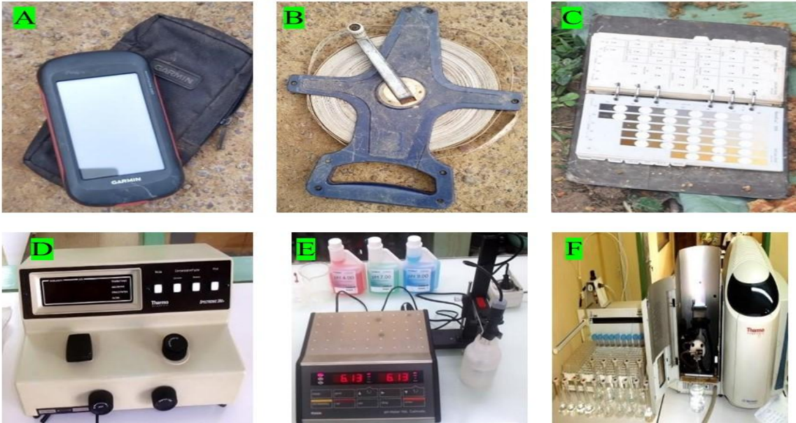
Figure 2. Soil prospecting and laboratory equipment. A: GPS, B: Tape measure, C: Munsel code, D: Spectrocolorimeter, E: pH meter, F: Spectrometer
