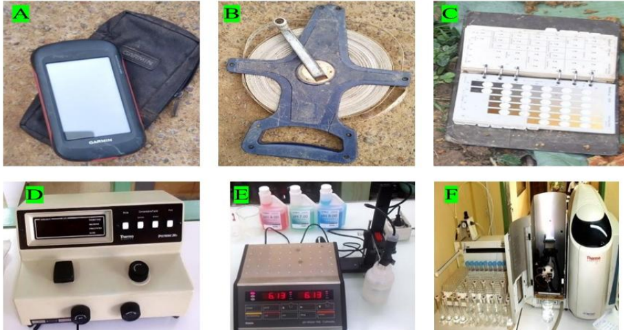
Figure 2. Soil prospecting and laboratory equipment. A: GPS, B: Tape measure, C: Munsell code, D: Spectrocolorimeter, E: pH meter, F: Spectrometer
