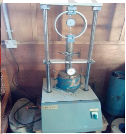
Plate 3: CBR Test set up
