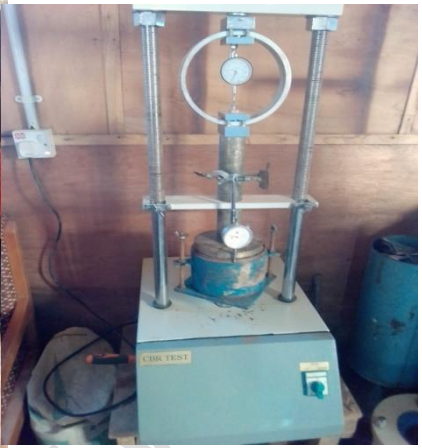
Plate 3: CBR Test set up
