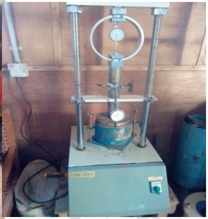
Plate 3: CBR Test set up
