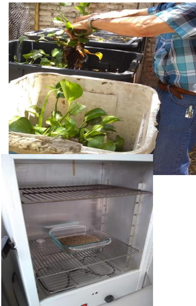
Fig. 4. Water hyacinth was dehydrated by sun exposition during 4-5 days; after, the semidry water hyacinth was cutting in small pieces and translated to laboratory for total dehydration using an Oven at 60-65 °C overnight.
