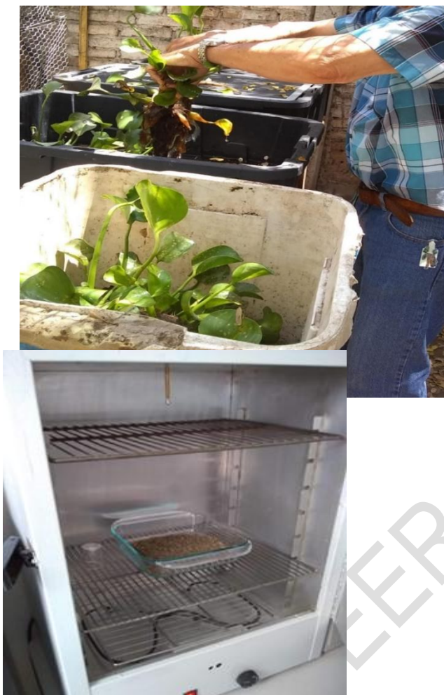
Fig. 4. Water hyacinth in preparation to be dehydrated by sun exposition during 4-5 days; after, the semidry water hyacinths were cutting in small pieces and translated to laboratory for total dehydration using an Oven at 60-65 °C overnight.
