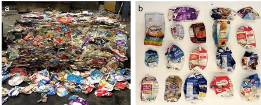
Fig. 4. Aseptic Packaging Container a) 2000 lbs. Bale, b) Material Content [15]
