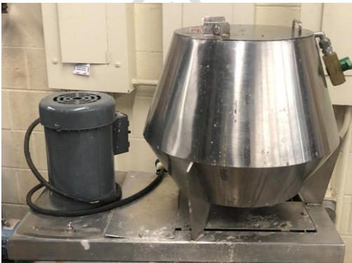
Fig. 5. Low Consistency Laboratory Repulper [33]
