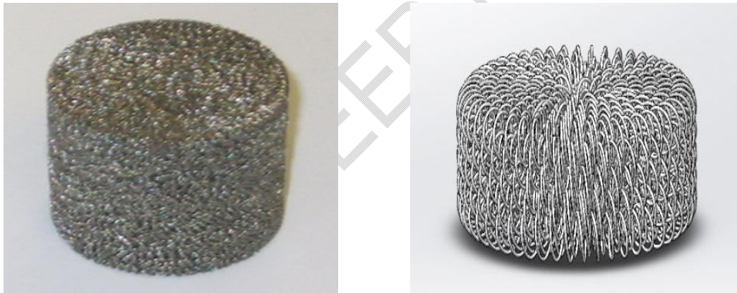
(a) A cylindrical metal rubber specimen (b) The constructed model of the specimen.
