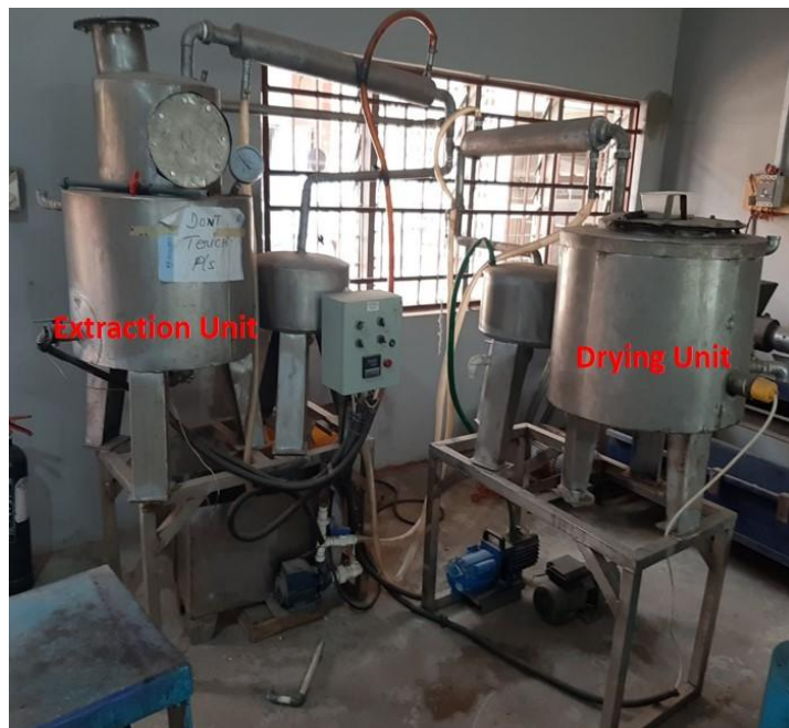
Figure 4. The macroscopic image of the fabricated natural dye extractor and dryer machines.
