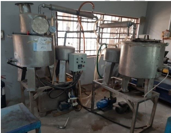
Figure 6. The macroscopic image of the fabricated natural dye extractor and dryer machines.
