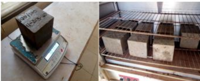
Fig. 7: Weighing and oven-drying of cube specimens.
