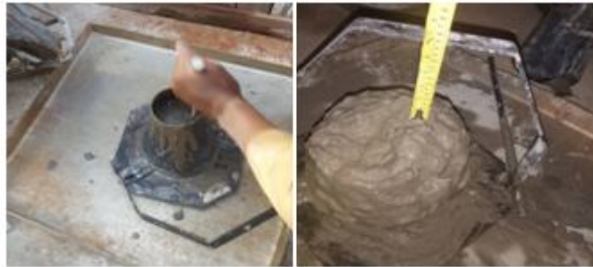
Fig. 5: Slump test being conducted on fresh concrete.
