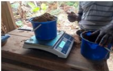
Fig 4: Batching process of the constituent materials.
