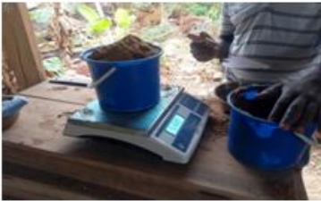
Fig4: Batching process of the constituent materials.
