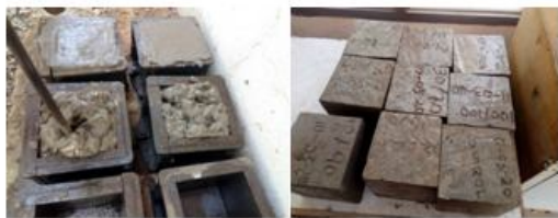
Fig. 6: Samples of cubes being moulded.
