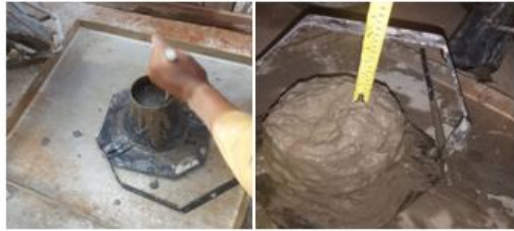
Fig. 5: Slump test being conducted on fresh concrete.
