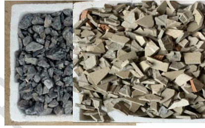
Fig 2: Sample of coarse granite aggregate used.
