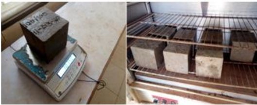
Fig. 7: Weighing and oven-drying of cube specimens.
