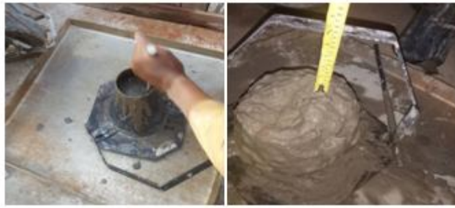
Fig. 5: Slump test being conducted on fresh concrete.
