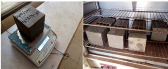
Fig. 7: Weighing and oven-drying of cube specimens.
