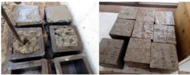
Fig. 6: Samples of cubes being moulded.
