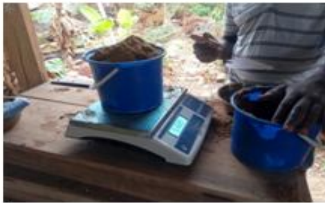
Fig 4: Batching process of the constituent materials.
