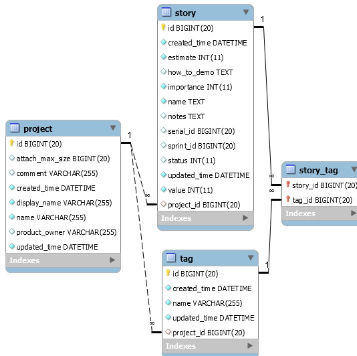
Figure 8 Entity relationship diagram of product backlog microservice table
