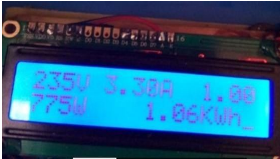
Figure 7: Snap shot of Prototype meter LCD display of voltage, current, pf, 'real-time' power and electrical energy
