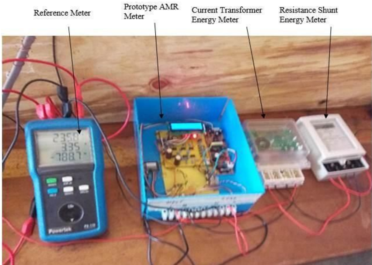
Figure 6: Electrical energy meters under test
