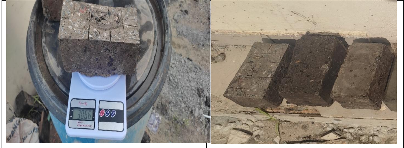
Fig.3. Interlocking paving stone made from waste plastics
