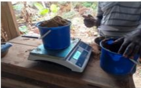
Fig 4: Batching process of the constituent materials.
