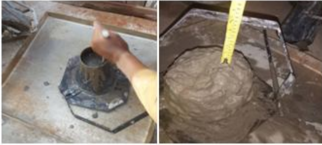
Fig. 5: Slump test being conducted on fresh concrete.
