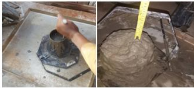
Fig. 5: Slump test being conducted on fresh concrete.
