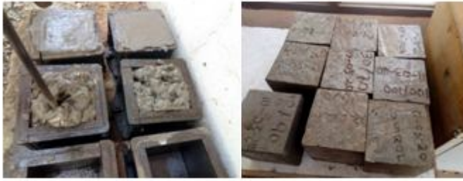
Fig. 6: Samples of cubes being moulded.
