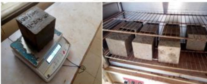
Fig. 7: Weighing and oven-drying of cube specimens.
