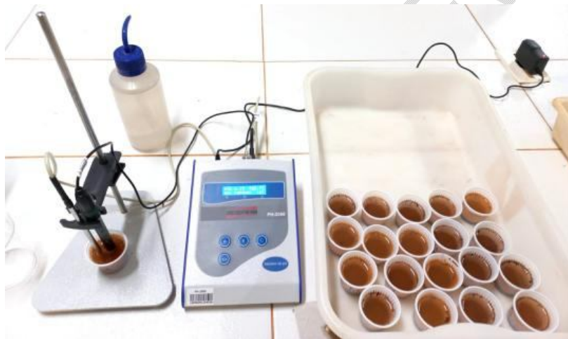
Fig.3. Determination of Oxisol pH in the soil laboratory of the Federal University of Rondonópolis, Rondonópolis-MT
