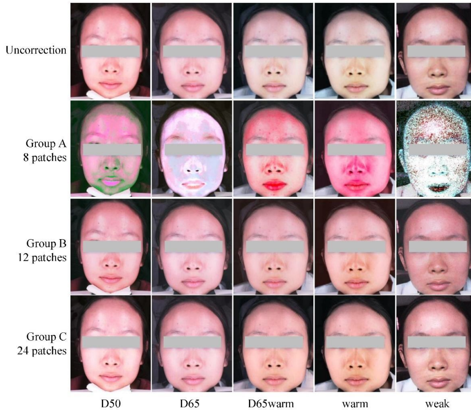
Figure 8 Sample results of facial color correction on Groups A, B, and C. From top to bottom: Groups A, B, and C, respectively. From left to right: D50, D65, D65warm, warm and weak.
