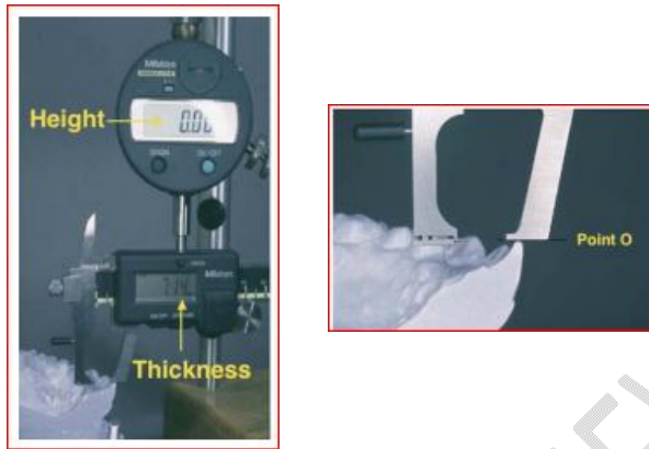
Fig. 7: The Electronic TARG has a precise measuring device that measures the distance (thickness) between the labial surface of the tooth and the slot of the bracket
