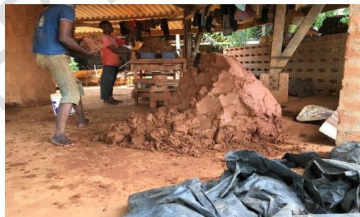
Fig. 5. Clay preparation and brick production
