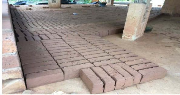
Fig. 6. Natural drying of bricks
