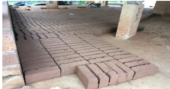
Fig. 6. Natural drying of bricks
