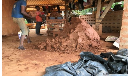
Fig. 5. Clay preparation and brick production
