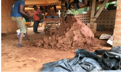
Fig. 5. Clay preparation and brick production
