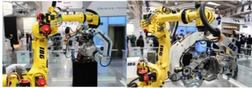
Fig. 15. Prototype of a robotized full-cycle and full-function automated passenger car transmission assembly system developed by IAG [70]
