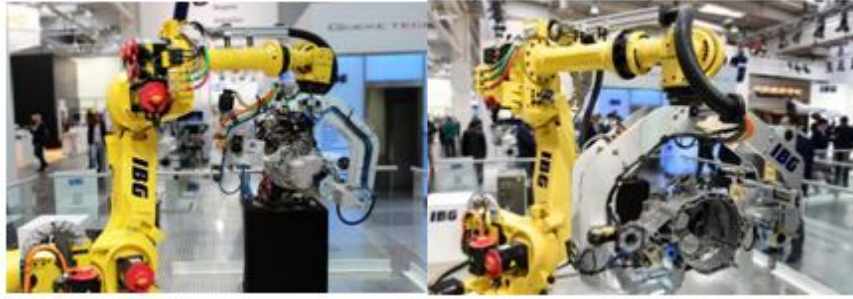
Fig. 15. Prototype of a robotized full-cycle and full-function automated passenger car transmission assembly system developed by IBG [70]
