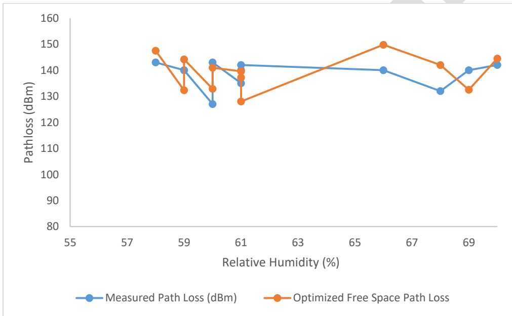
Figure 8: Graph of Measured/Optimized Free Space Path Loss against Relative Humidity
