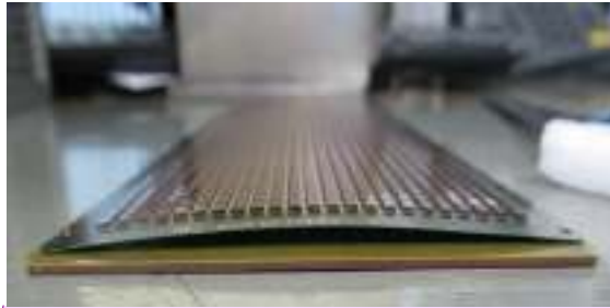
Fig. 1. Warpage visible on substrate after oven curing
