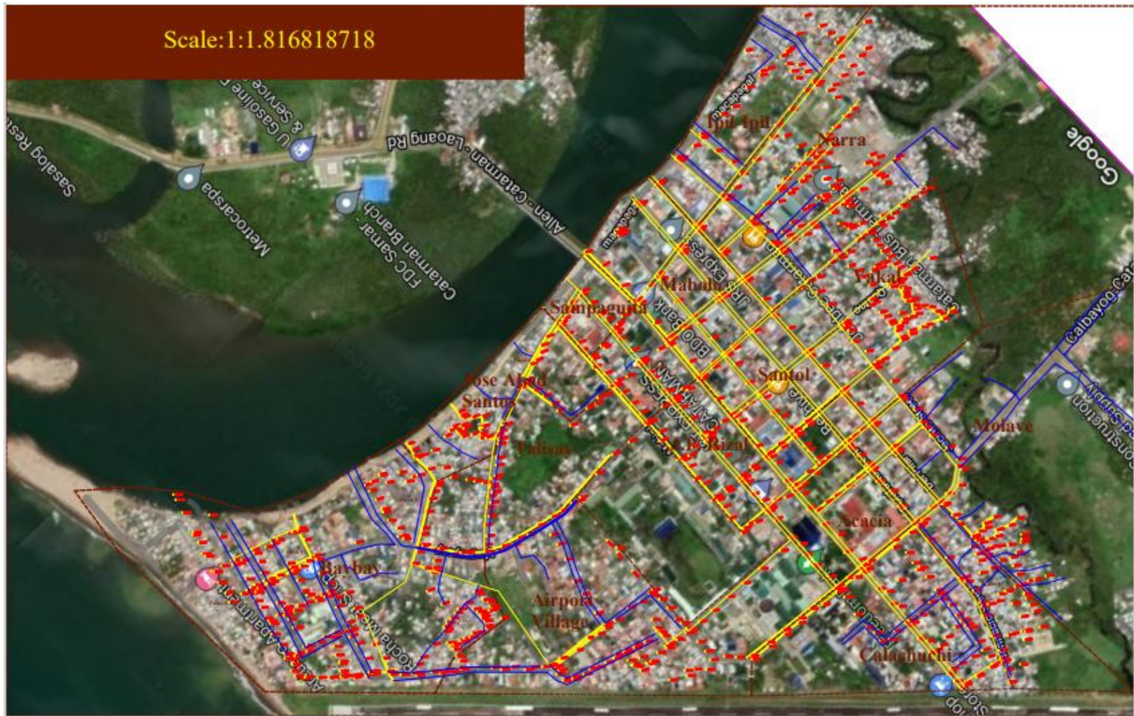
Figure 1. Catarman, Northern Samar Drainage Canal System Map Note: Yellow colored Lines are the existing drainage canals; Blue colored lines are the required additional canal.
