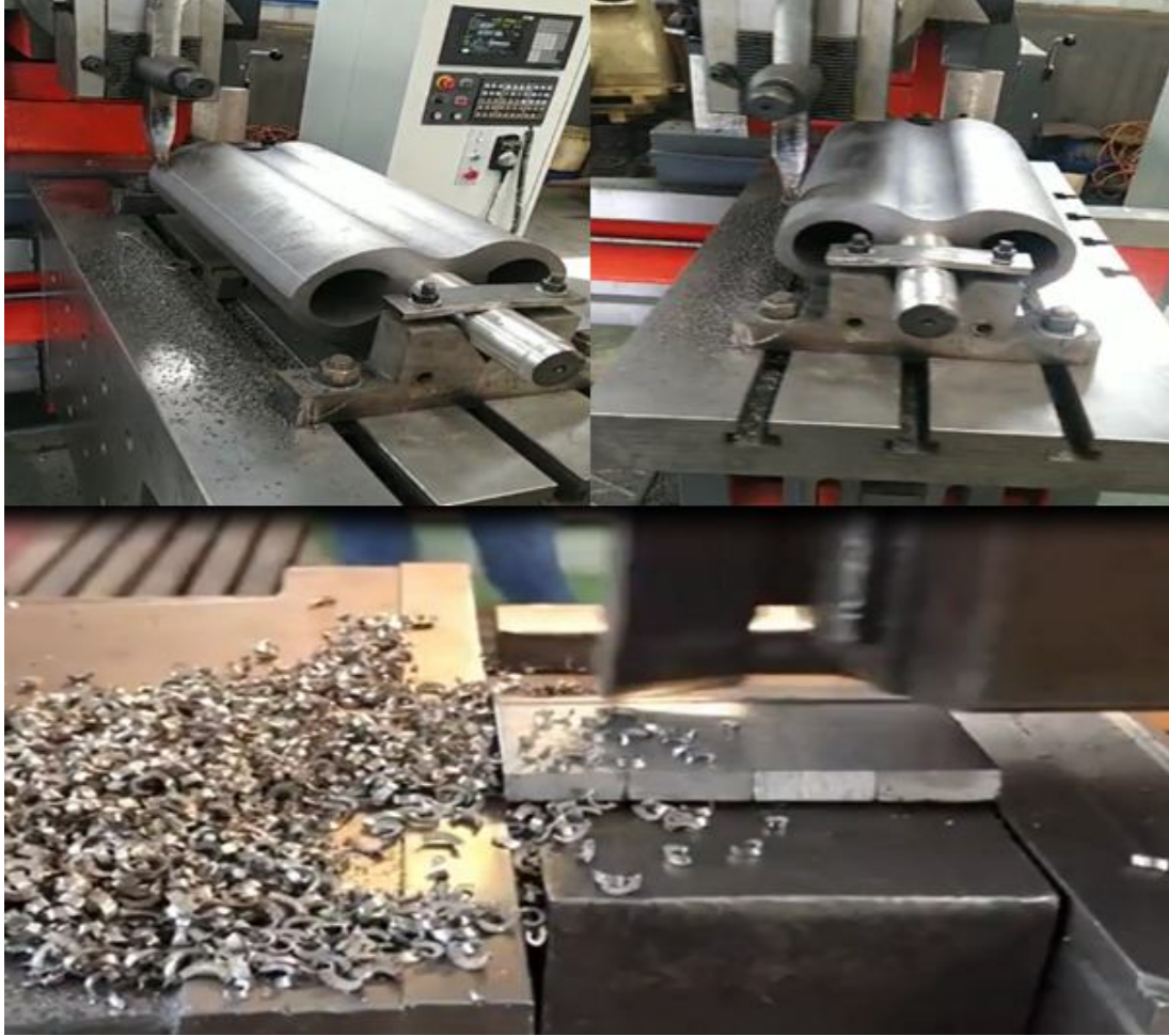
Fig. 5.2-axis CNC shaping machine vs single automatic x-axis conventional shaping machine
