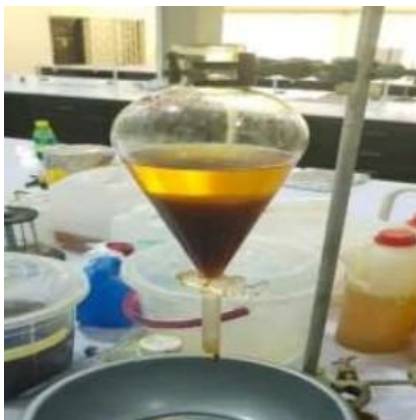
Fig. 3. Azelia bella oil Biodiesel separation.
