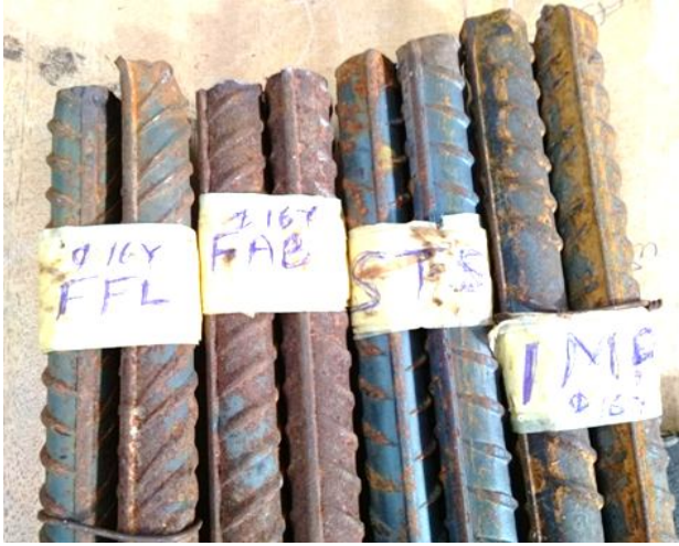
Fig 1: Typical samples of reinforcing steel bars in Ghana
