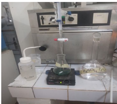
Figure 2: Dosing of the distillate and turning of the solution
