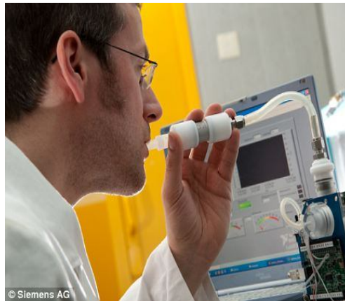
Fig. 2. Siemens device for measuring the amount of nitrogen monoxide
