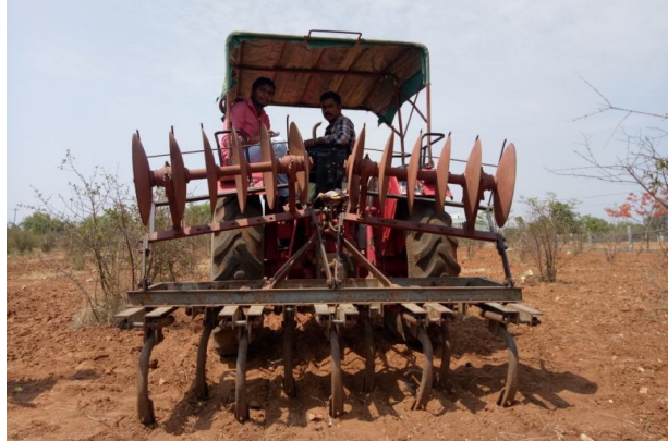
Fig. 3: Testing of developed combination tillage implement
